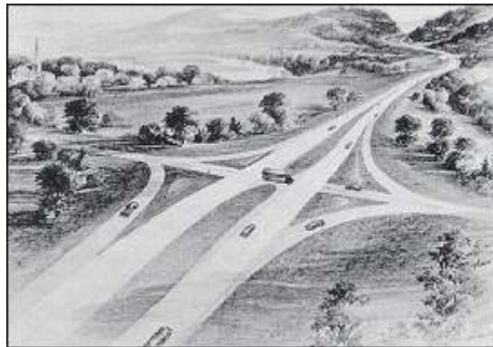
Artist's conception of an interstate highway with at-grade crossings on a four-lane highway designed in conformity with the standards approved in 1945.
